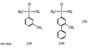
The substitution of a second methyl group ortho to the p-phenyl substituent produces an additional loss of the electronic contribution of the phenyl substituent (11). Thus there must be substantial deviation from coplanarity of the rings.
